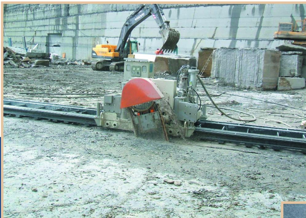
Fig.1 Super Jet Belt 950 in taglio verticale / Super Jet Belt 950 during vertical cutting
