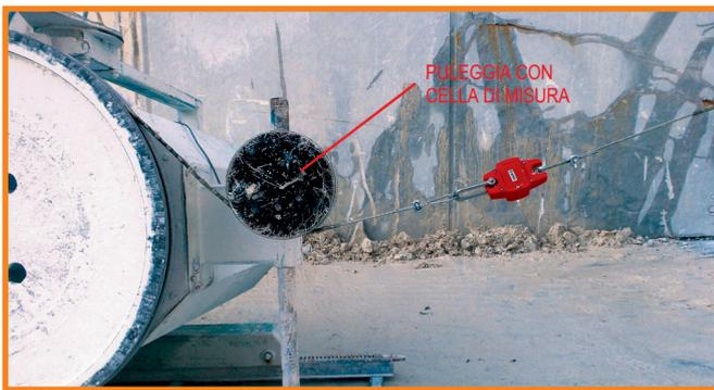
Fig.5 Taratura con dinamometro / Calibration with a dynamometer
